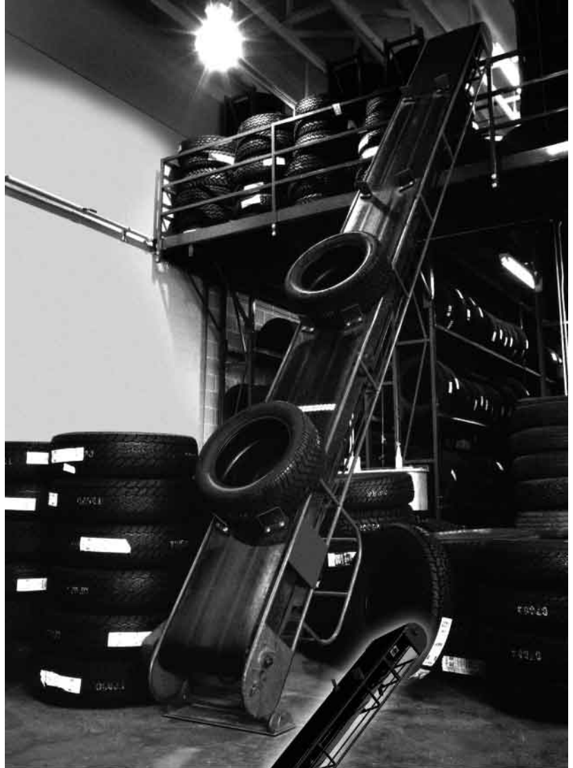
Portable stand w/hand winch adjustment
